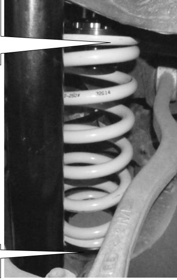
Use the supplied spring support at the bottom end of the spring.
