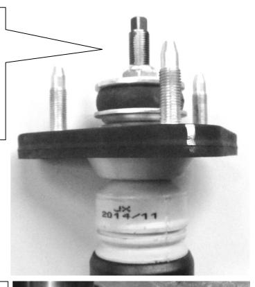
Mount the rear axle adjustment between spring and chassis, the original spring support is no longer used. You have to remove the rear axle adjustment to correct (screw up the threaded ring) the car height. Attention: Before the installation of the height adjustment perch the touching surface area have to be cleaned.
