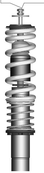
Tightening torque for the piston rod nut is 20 Nm (15 ft-lb). The strut unit has to be installed according to manufacturers recommended settings regarding tightening torque and fixing specifications.
